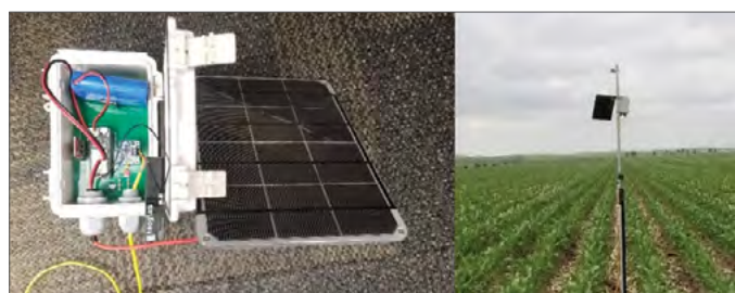
Figure 2. IoT device for measuring surface temperature (left) and the device deployed in a field (right).
