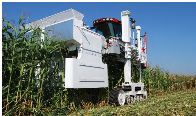
Figure 8. Corteva Agriscience's Boreas wind machine creates winds that can exceed 100 miles per hour to test for standability in corn hybrids.
