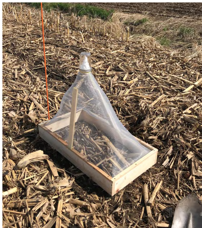
Figure 10. Trap set up following soybean planting to measure soybean gall midge adult emergence from the soil in 2019.
