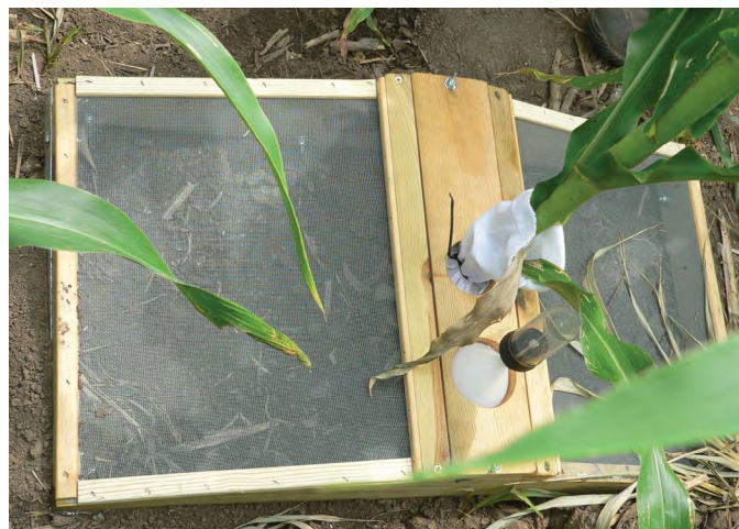
Figure 2. Emergence cage used to capture corn rootworm adults emerging from the soil.
