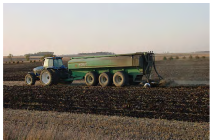
Figure 4. Increasing the number of axles carrying a heavy load increases the surface area of contact and reduces maximum axle load but also increases the number of times pressure is applied to soil in the wheel track.
