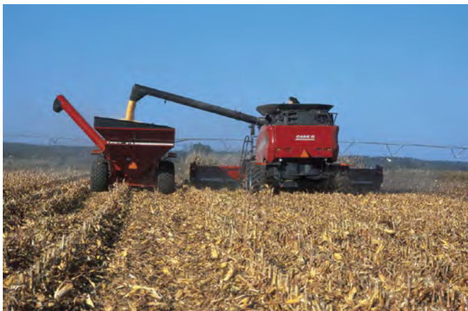
High axle loads of large agricultural machines, such as tractors, combines, and grain carts, can create compaction deep into the soil profile when operating in wet conditions.
