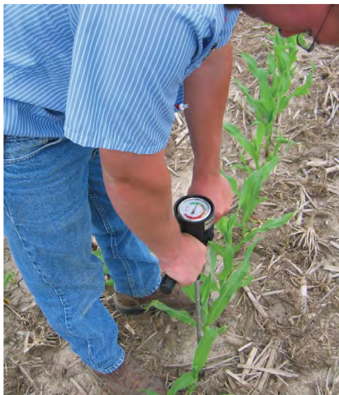
Figure 8. Measuring soil compaction with a soil penetrometer.
