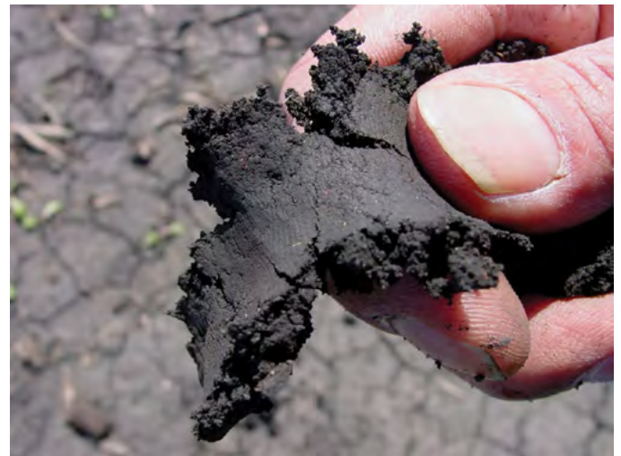
Figure 5. The “ribbon test” can be used to assess soil moisture and determine if soil is at high risk for compaction.
