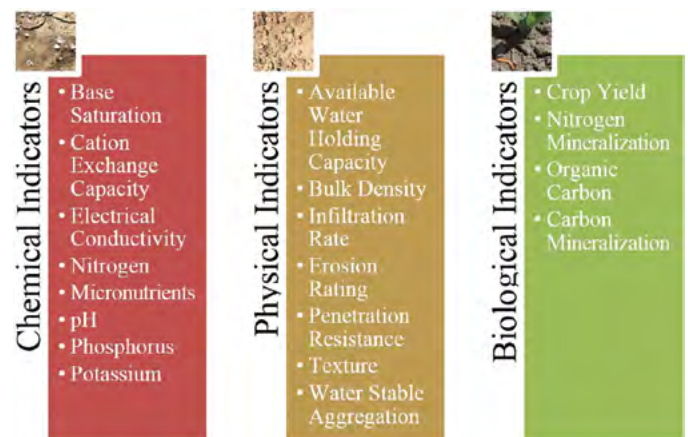
Figure 1. Chemical, physical, and biological indicators designated as Tier 1 Soil Health Indicators by the Soil Health Institute.
