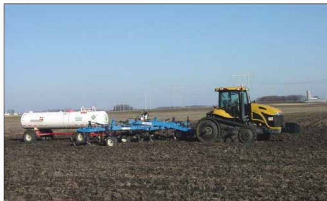
Figure 1. Tractor pulling a field cultivator and an anhydrous ammonia tank.
