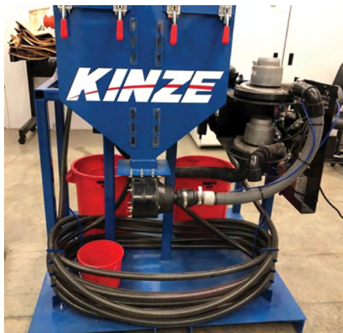
Figure 5. This bulk fill test stand was developed by Kinze Manufacturing to replicate their air seed delivery system. The system includes a small bulk fill chamber, entrainer, seed delivery tubing (length equivalent to a 24-row planter), and two individual vacuum meters.
