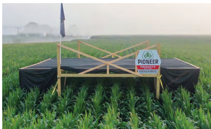
Figure 1. Shade structure that was used to apply reduced solar radiation treatments.
