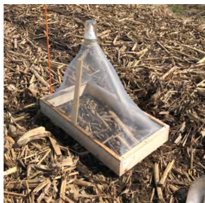
Figure 8. Trap set up following soybean planting to measure soybean gall midge adult emergence from the soil in 2019.
