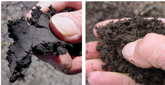
Figure 1. (Left) Soil that is too wet to plant, as it forms a ribbon when squeezed between your thumb and forefinger. (Right) Soil that is fit for field work when it crumbles when pressed.
