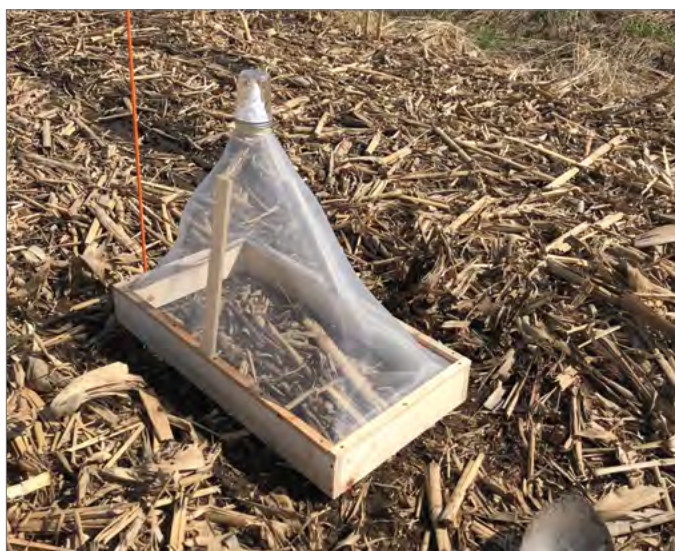
Figure 9. Trap set up following soybean planting to measure soybean gall midge adult emergence from the soil in 2019. Photo courtesy of Lauren Botine, Corteva Agriscience Agronomist.
