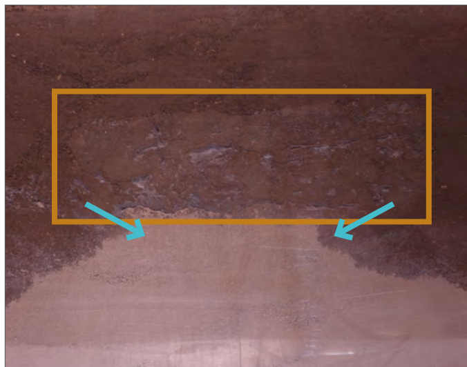
Figure 9. Water as it drains through the soil profile is limited by a zone of highly compacted soil (outlined by the orange box). Water drains through less compacted soil more quickly and eventually begins to move below the zone of high compaction (blue arrows).
