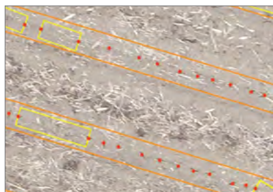
Figure 4. Corteva Agriscience image analysis software is able to detect individual plants (marked with red dots) and gaps in stand (marked with yellow boxes), providing a robust characterization of stand establishment.
