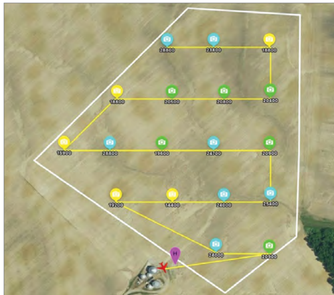
Figure 5. A typical stand evaluation flight plan showing 18 1/10 acre sample points distributed throughout the field.
